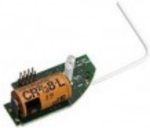
RadioLink module Ei600MRF, Lithium 3V 10 years battery Kurzbeschreibung Learn More
