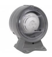
Air duct construction set for using IQ8Quad OT LKM. Suitable for application in air ducts with widths between 140mm and 2700mm. The operation status of each detector is externally displayed. The detector can be maintained without opening the housing. Air flow indicator for indicating air current. Optional filter for application in contaminated environments.
